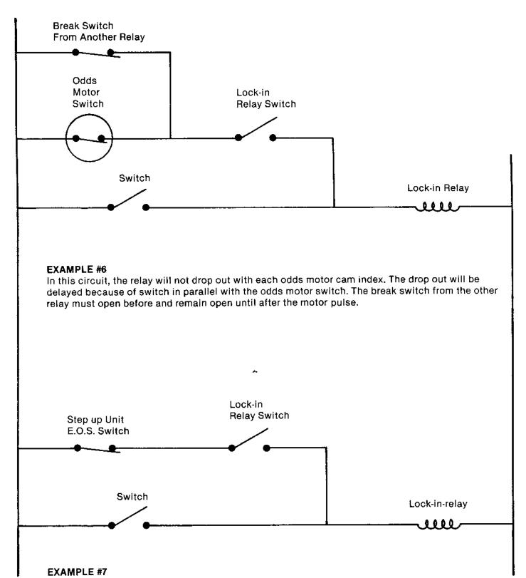
The relay is locked in through a step up unit end of stroke switch. The step up unit must advance for the relay to drop out. A typical example of this circuit is in the odds relay lock-in circuit.
