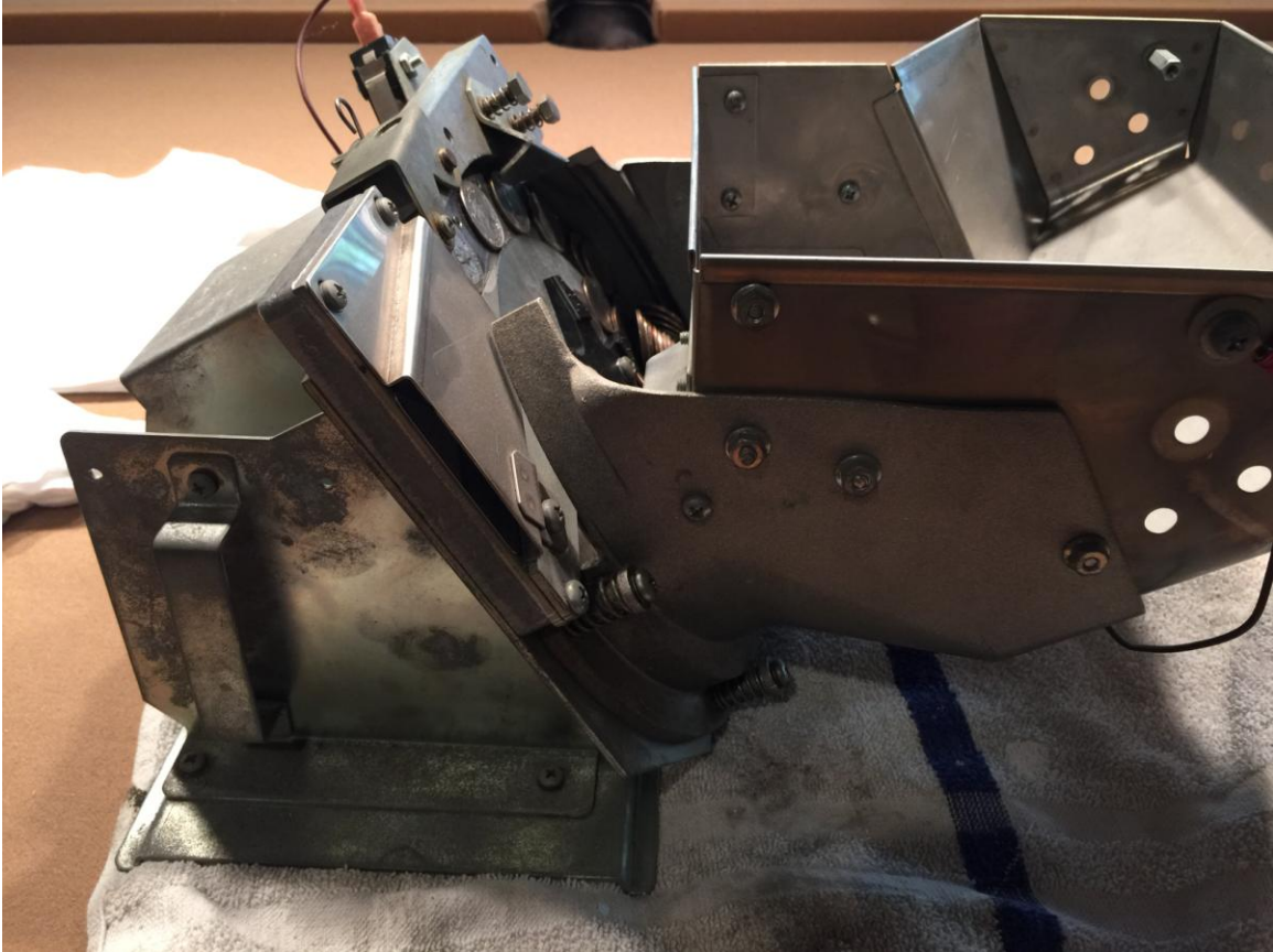
Side view of hopper - remove the hopper only by grasping the handle shown
