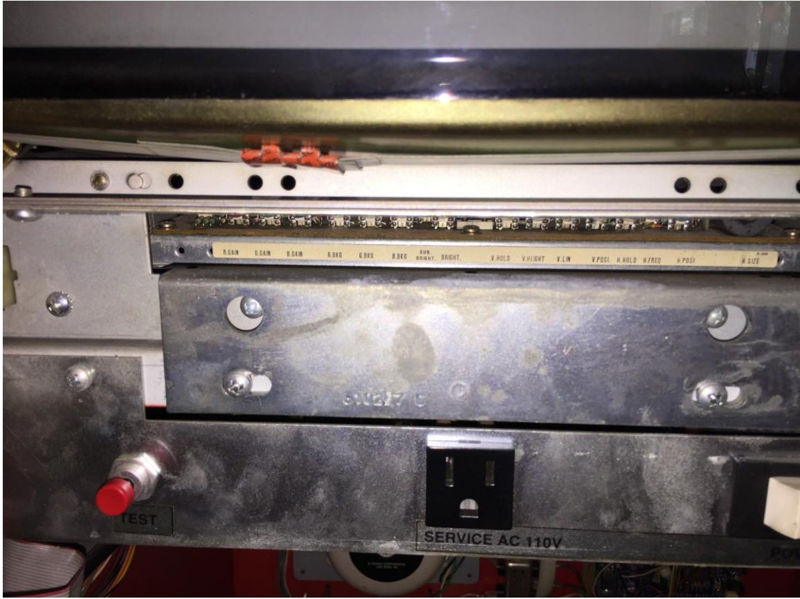
Video screen adjustment labels - Red Gain, Green Gain, Blue Gain, Red Blanking, Green Blanking, Blue Blanking, Sub. Bright, Bright, Vertical Hold, Vertical Height, Vertical Line, Vertical Position, Horizontal Hold, Horizontal Frequency, Horizontal Positioning, Horizontal Size
