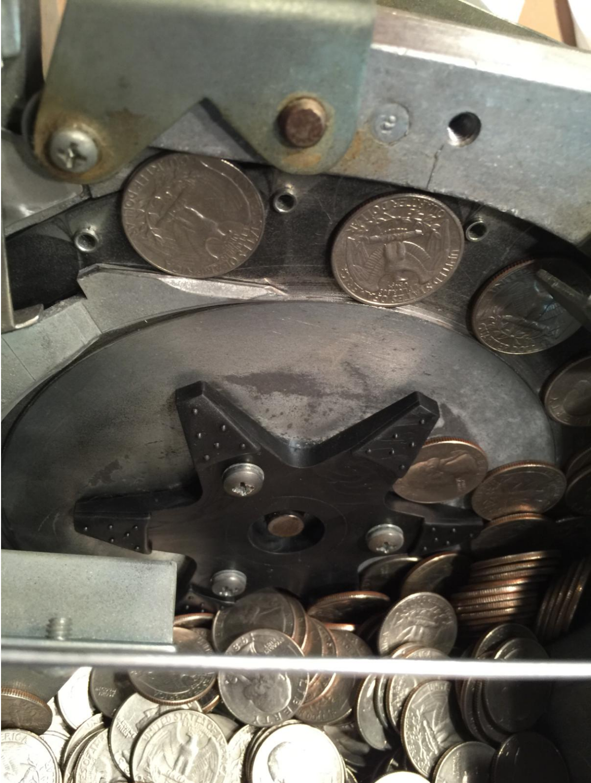
Close-up view of hopper agitator - replace this every two to three years
