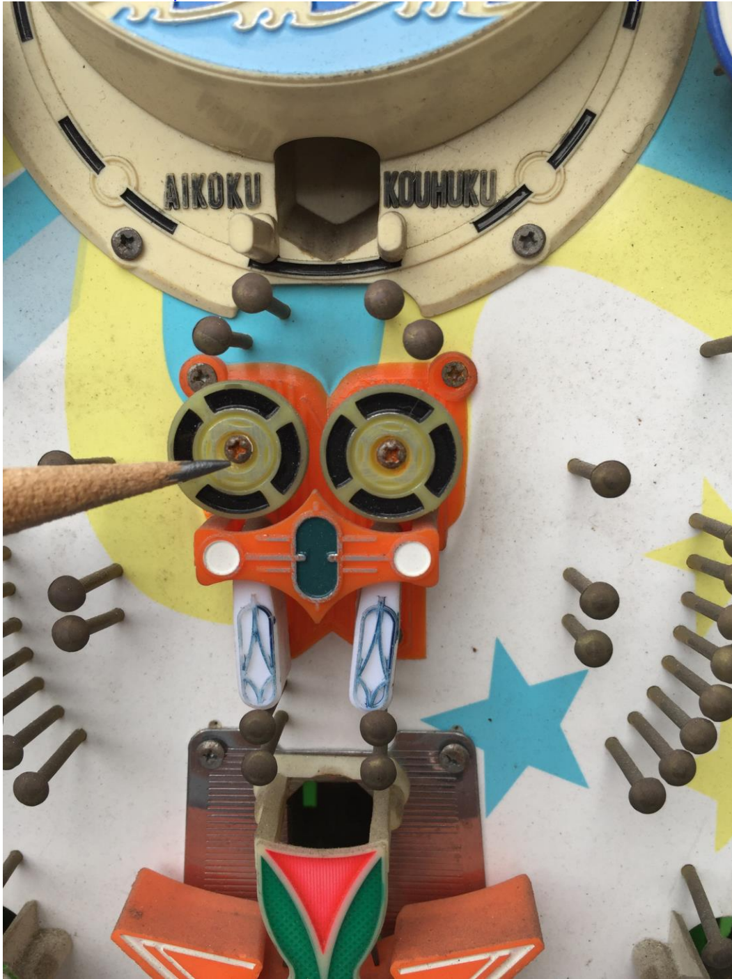
Ball Entrance - (just below the main reward pocket; a ball enters, slows down due to the "fins" at the exit and then it enters the next reward pocket)
