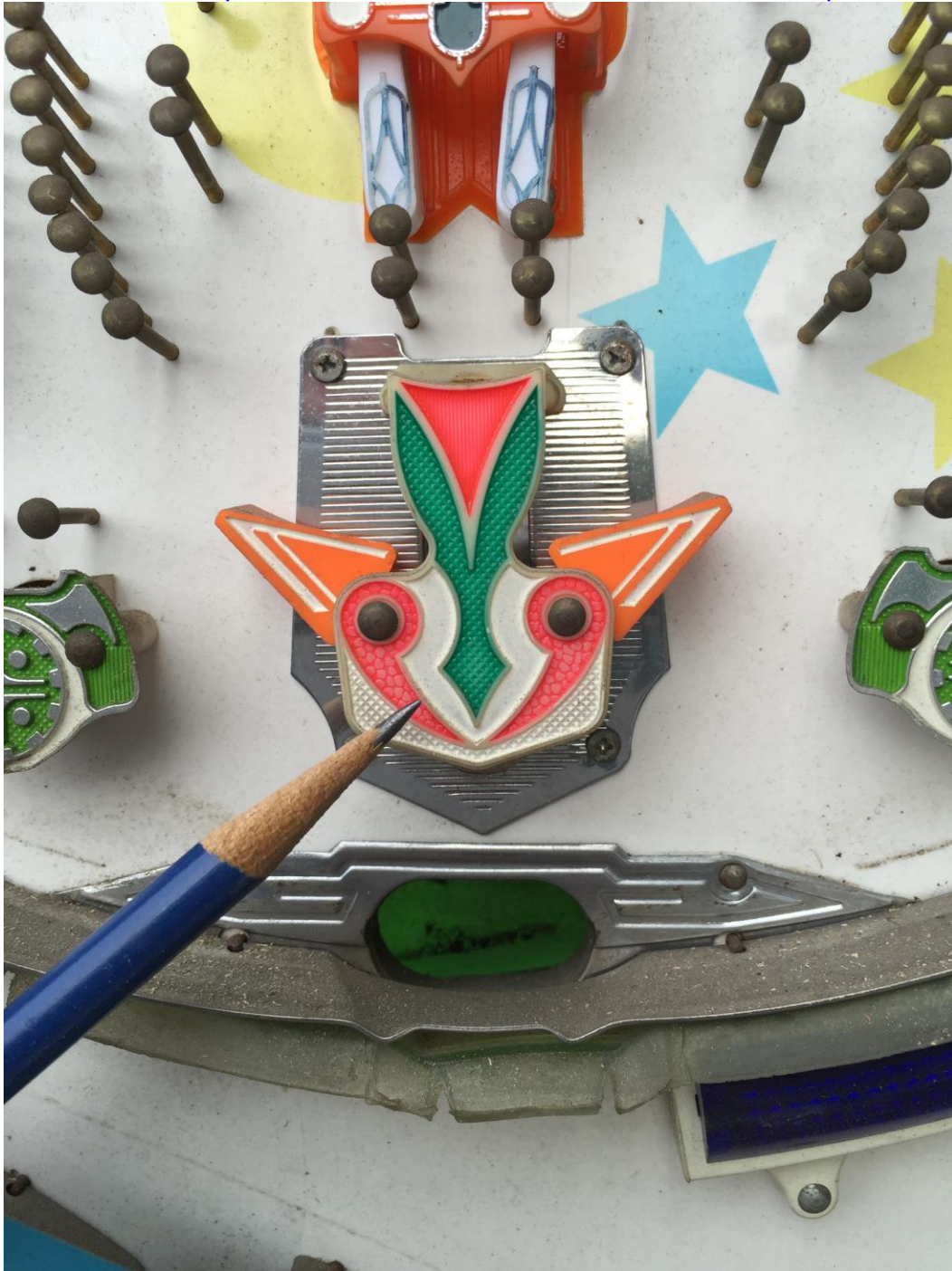
Reward Pockets - (these open and close when a ball enters; keep clean, lubricate the hinges)
