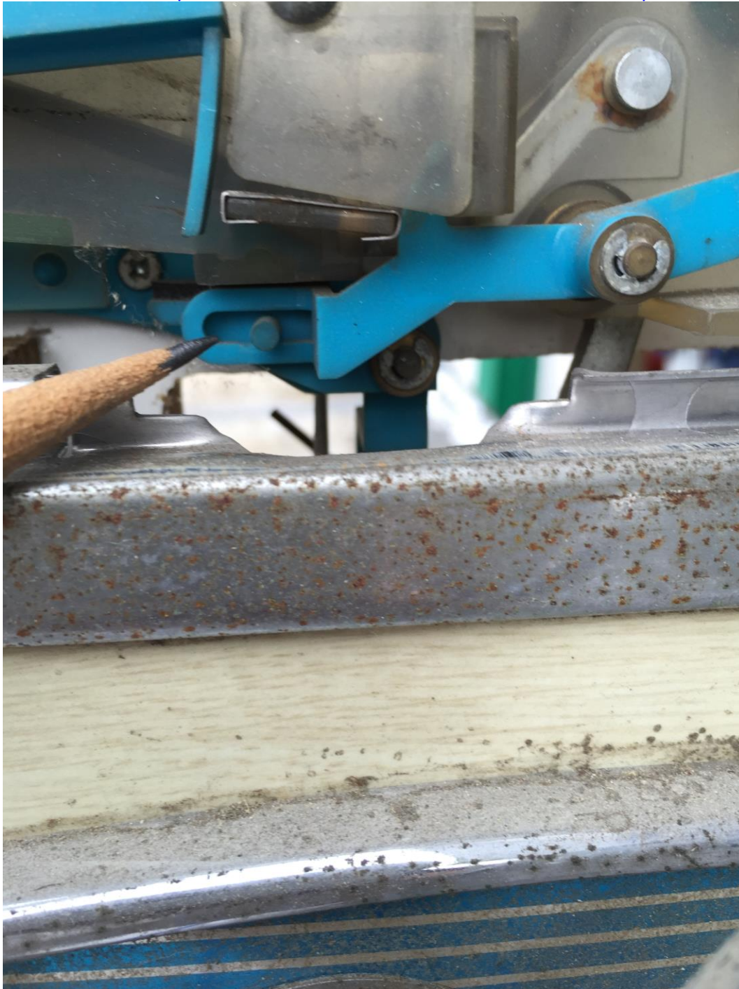
Pivot - (allows blue lever to slide; keep clean and lubricated with silicone)
