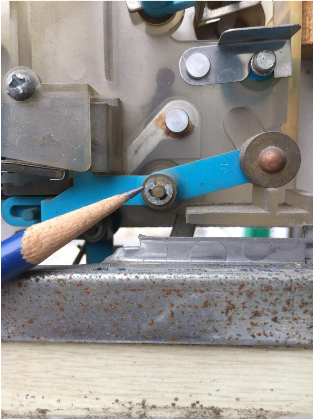
E-clip and Counterweight - (use silicone spray here)
