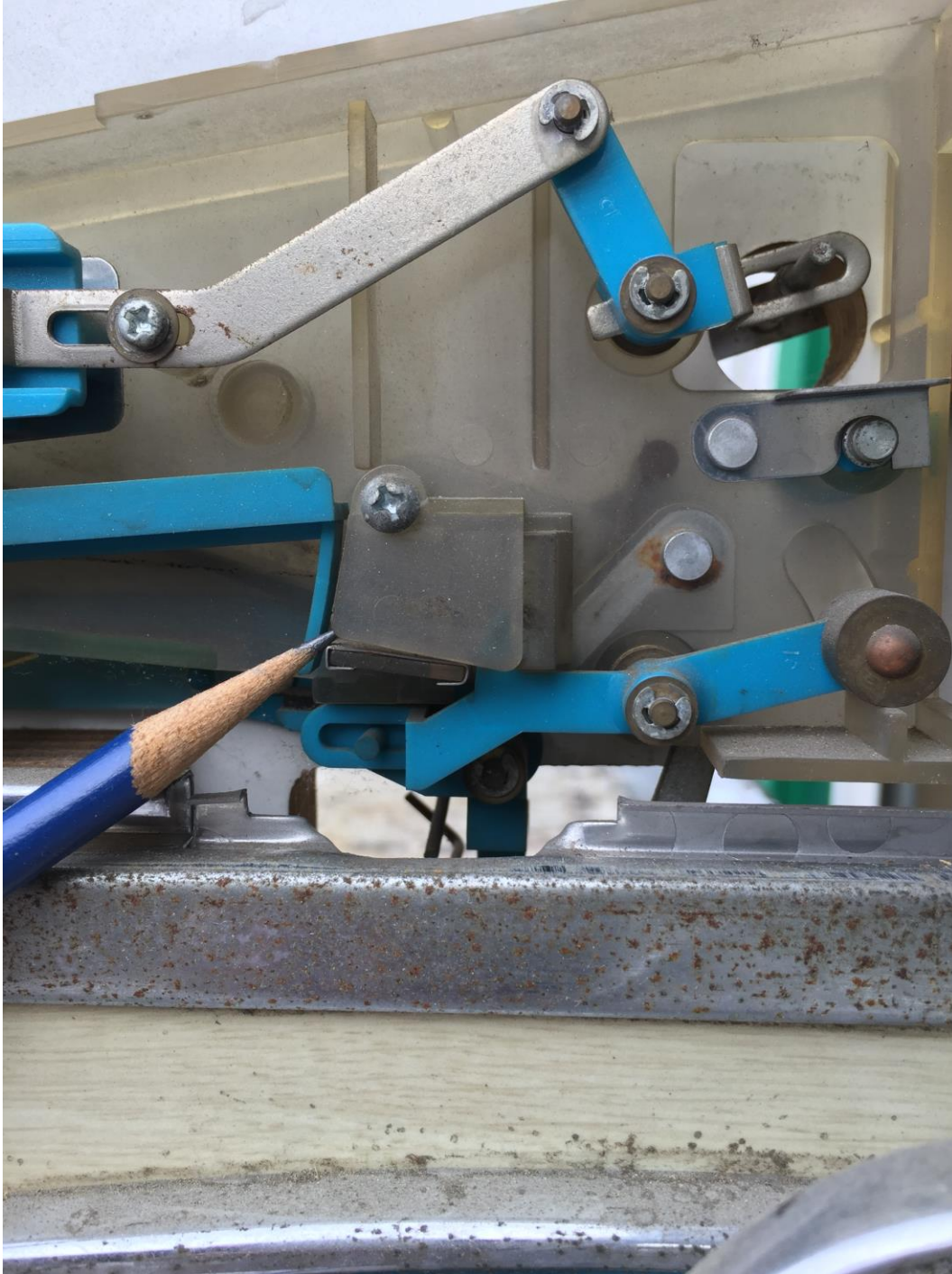
Ball Entry Holding Area- (this shield prevents the ball from falling out of its intended path; keep this and the blue plastic path clean and smooth; the ball bearing enters into this chamber in preparation to be launched by the spring-loaded mallet in back)
