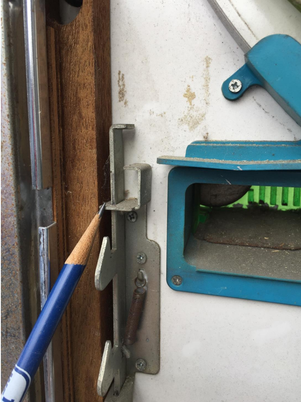
Latch Release Assembly - (on front of game below main glass door; push lever down to release the ball recovery assembly just below this latch)
