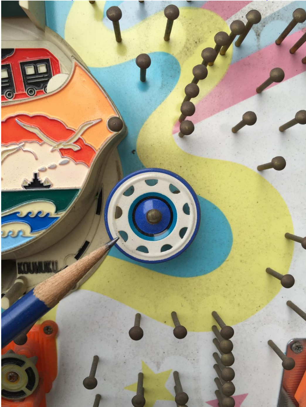
Spinner - (these rotate quickly when a ball strikes the mechanism; keep clean and lubricated)
