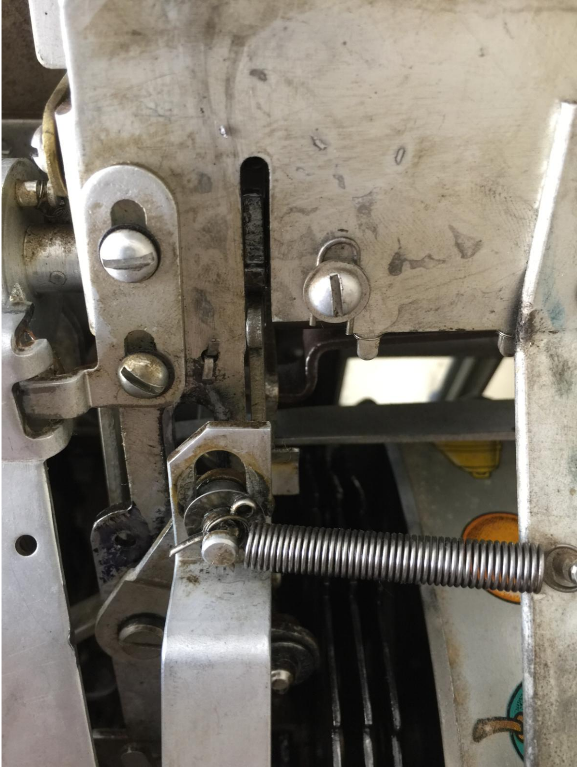
Spring attached from support bracket to timing lever. Oil this spring lightly to prevent rust.
