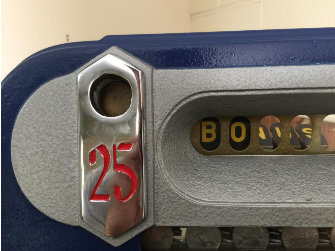
Outside view of annunciator window with the escalator filled with coins beneath it.
