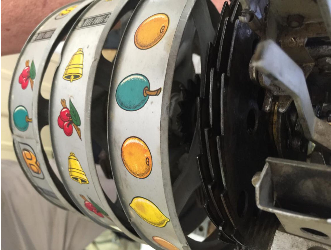
Closer view of the letter "B" on reel number 1 in line with roller bearing. The vertical payout pushback lever (gray color) is visible to the upper middle right. The coin tube entrance is at the lower right.
