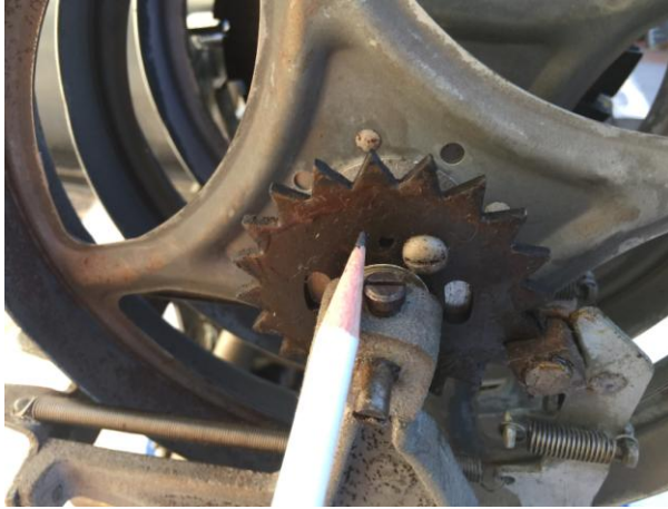
1 of 3 gears (on reels) for indexing
