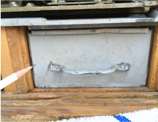
Coin Box - (inside of casing)
