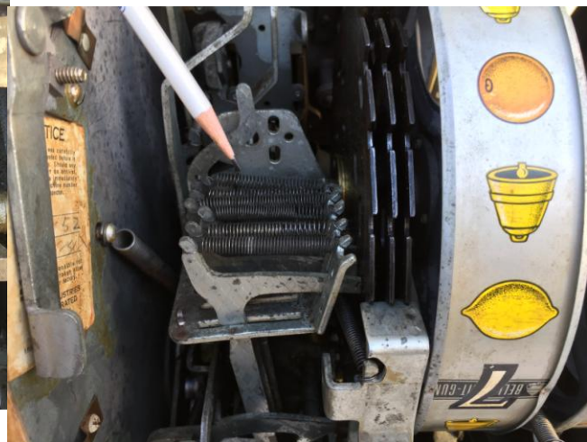
Vertical Payout Levers - (to the left of the drilled Reel Discs)
