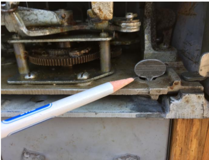
Thumbscrew, or bolt - (holding mechanism to casing)
