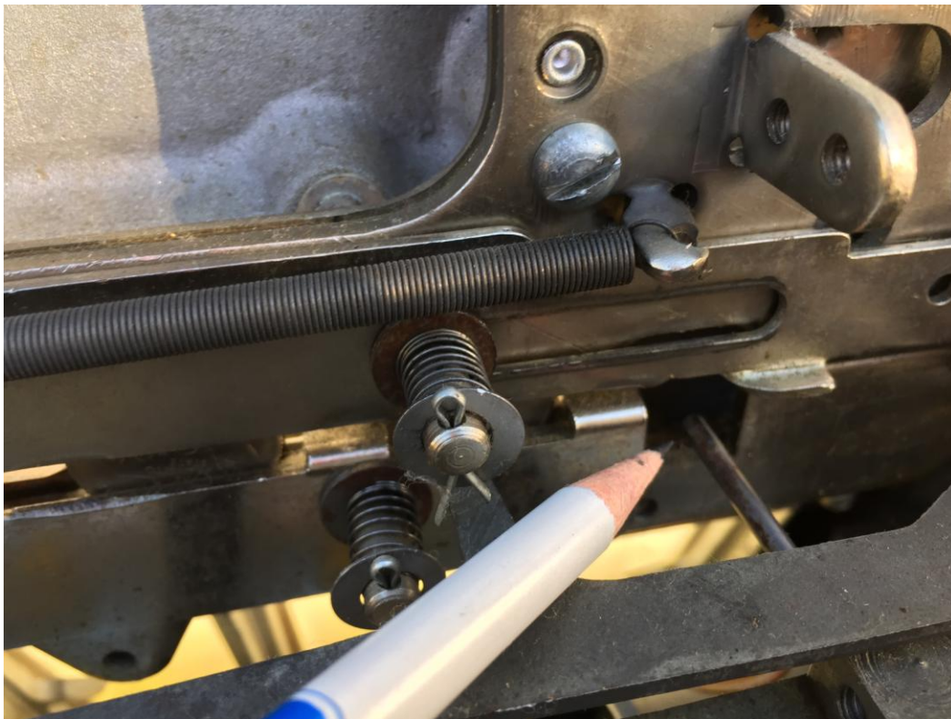
Sensing Pin - (coin rests against tip to allow handle to be pulled)
