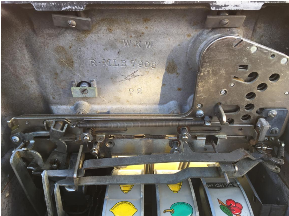
View of: genuine MLB part number, Escalator, Sensing Pin, Coin Detector Lever Assembly - (bottom lever), Check Detector Lever - (top lever)
