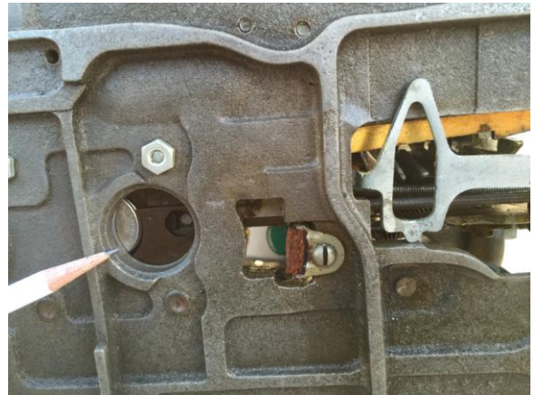
Safety Slide controlled by "Tilt" Lever
