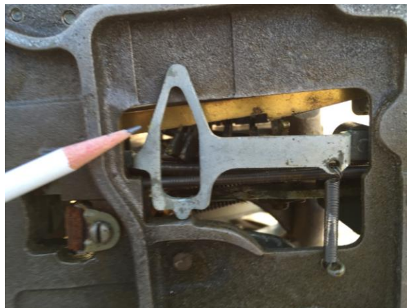
Safety Slide Lever Assembly - ("Tilt" Lever)
