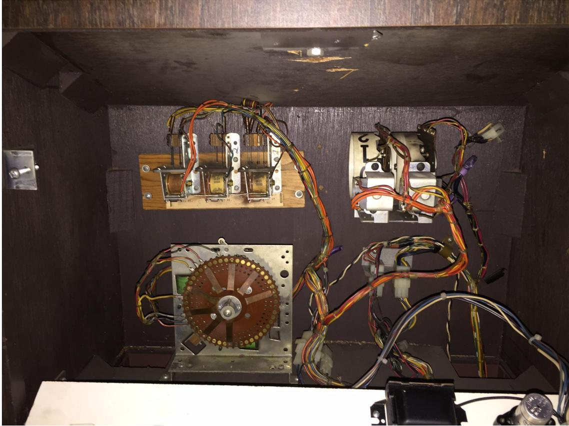
Stepper Switches, Coils, Relays, Transformer, Starter, Counter, Wire Harnesses, Molex Connectors - (these components are used for a three-coin 1090 dollar machine, all of this is housed behind the fluorescent lamp assembly)
