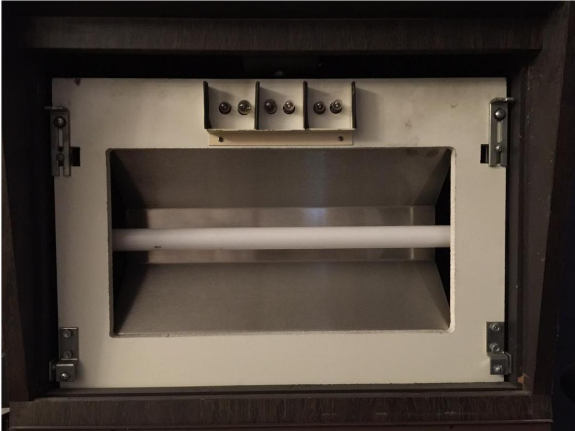
Fluorescent Lamp Assembly - (secured by two friction brackets; DO NOT tighten these screws! - they must be 'loose' to allow the owner to slide up/down allowing access to the steppers and relays inside; over time, replace the incandescent bulbs with LED 6 volt bulbs)
