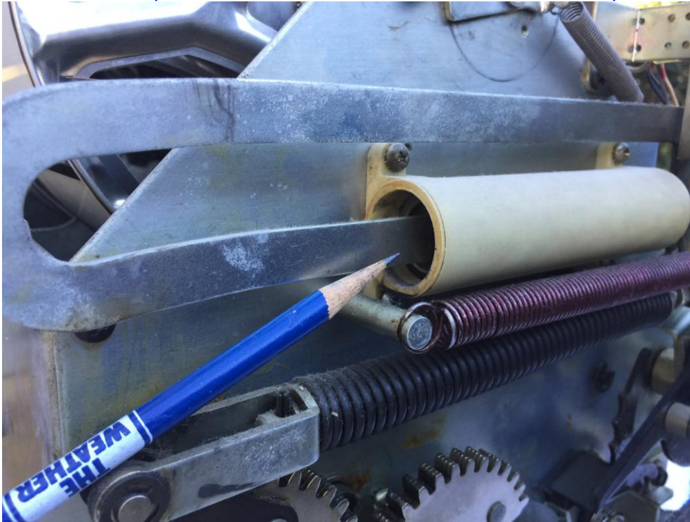
Air Cylinder of Dashpot Link and Pin Assembly - (piston, and neoprene piston cup seal inside)
