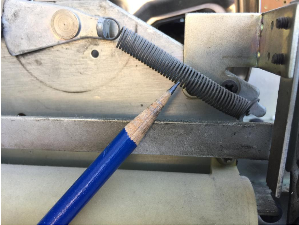
Reel Lock Lever Right - (attached to a spring; there are two such levers a left lever, and a right lever)
