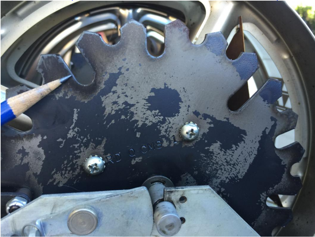
Index Plate on Reel Assembly - (with radial, variable-depth cuts)
