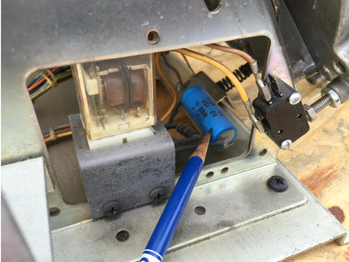
Electrolytic Capacitor - (50 mfd at 50 volts; replace this capacitor every 5 years, be sure to observe correct polarity!)
