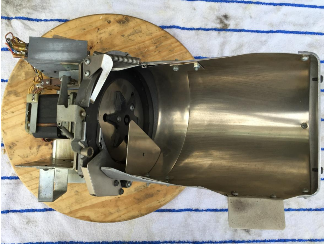
Top View of Hopper - (called a "snow hopper" in Bally machines after 1976)
