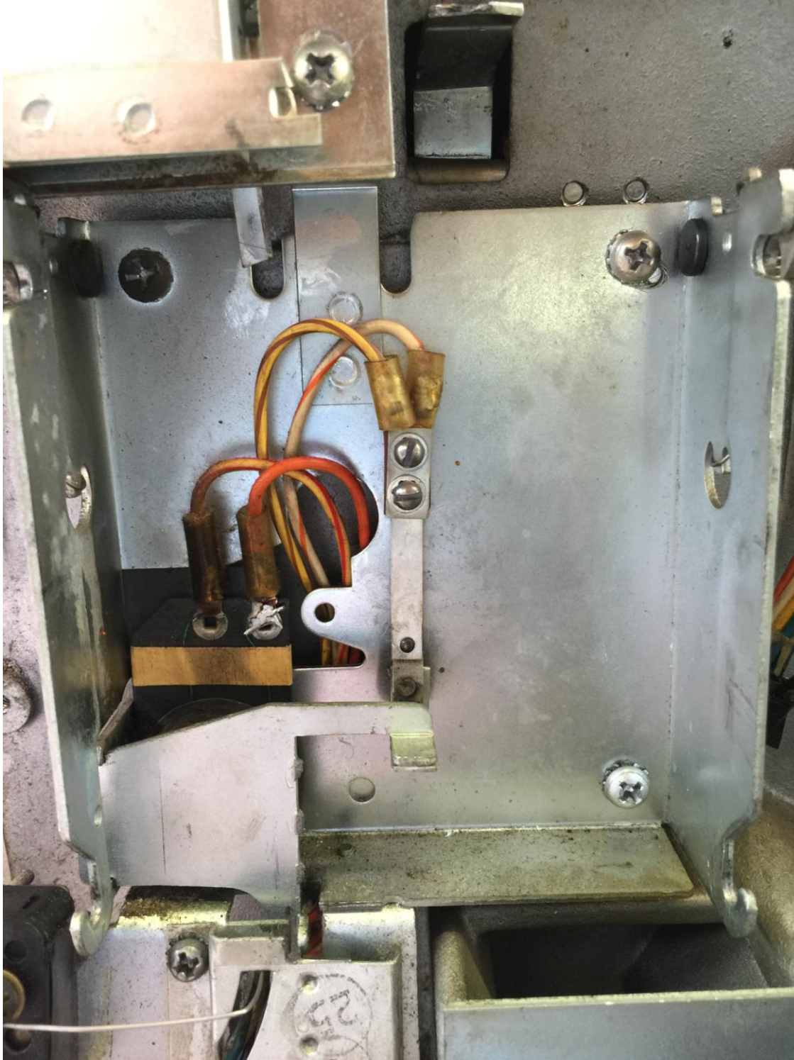
Coin Lockout Coil - (directly behind the coin-mech; keep this coil and plate clean by using contact cleaner - DO NOT USE "water displacement" type sprays)
