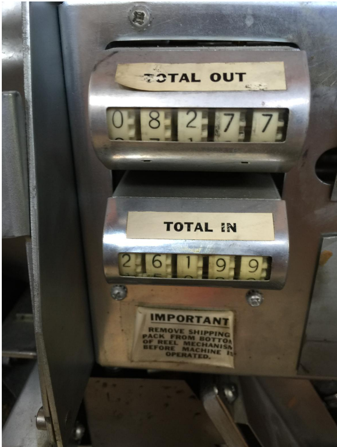
Total Out/Total In Meters - (these are attached on the front of the reel assembly for this particular machine - 742A)
