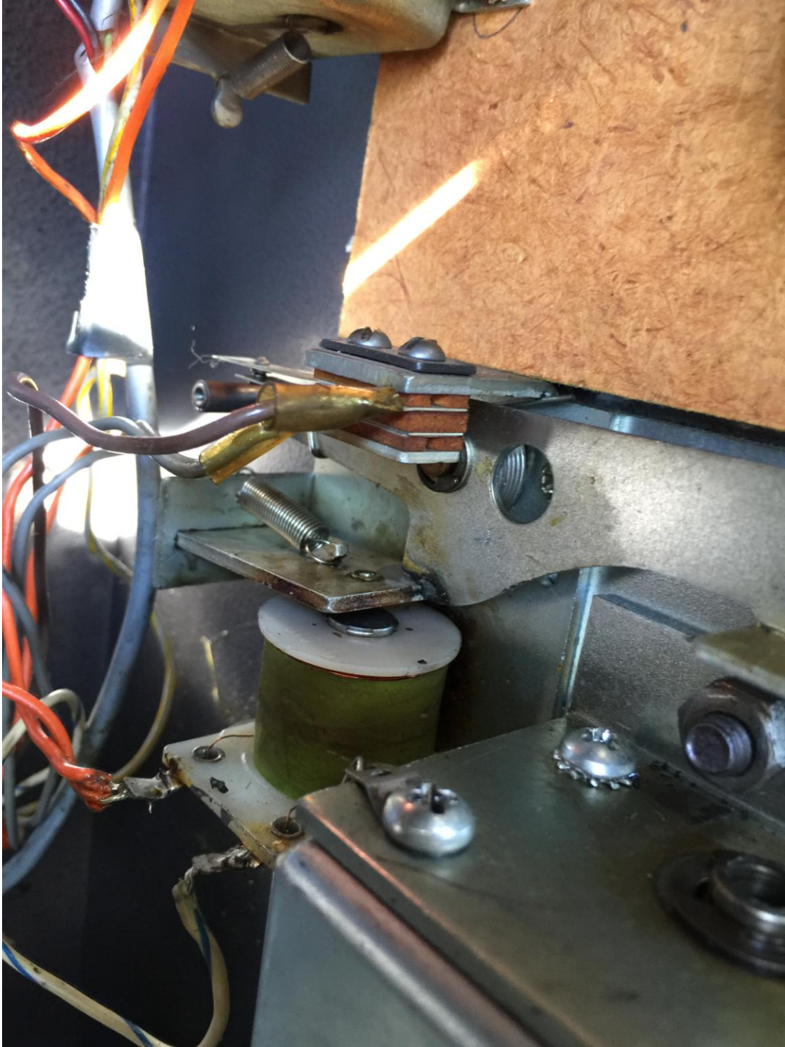
Solenoid - (triggers to allow handle to be pulled by slot player; keep this plate and the contacts clean with contact cleaner, clean the relays above it as well)
