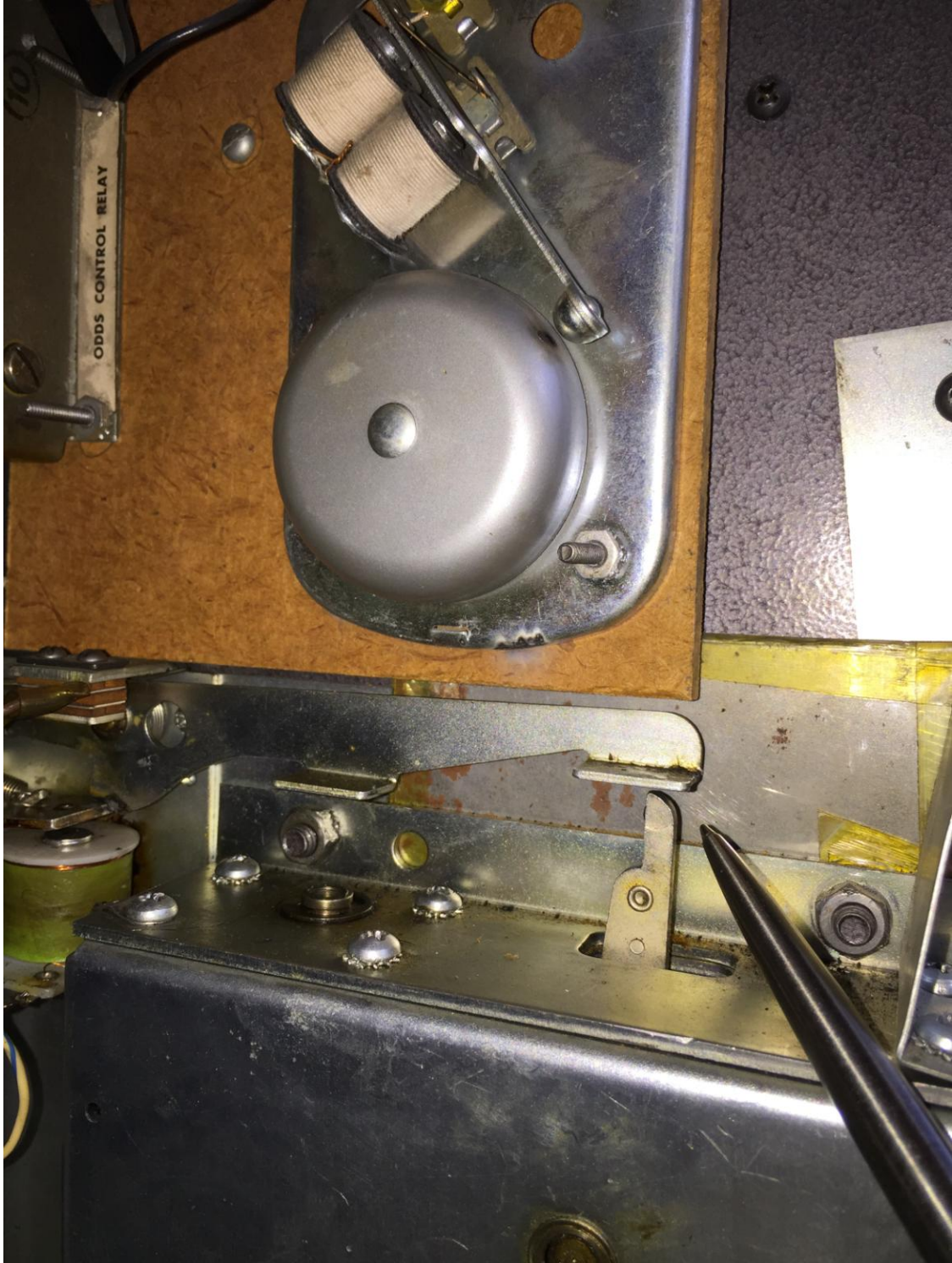
Bell, Release Pawl, Handle Release, Coil, Odds Control Relay - (interior right hand side of the machine)
