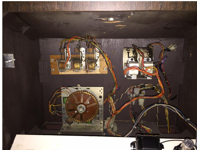
Stepper switches in upper cabinet
